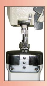
HIGH SPEED **POST TYPE** TWO NEEDLE ANGULAR STITCHING (SPLIT NEEDLE BAR) DROP FEED, NEEDLE FEED **WALKING FOOT ALTERNATING PRESSER FEET** LOCKSTITCH MACHINE
